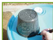
Trace a hole for the basket
