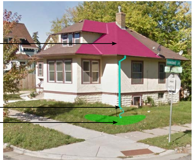
Raingarden capturing specific part of roof
